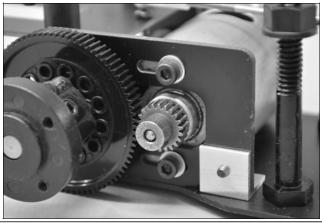
STEP 21 INSTALL YOUR MOTOR WITH TWO SCREWS AND WASHERS PROVIDED. SLIDE THE PINION GEAR ONTO THE SHAFT AND LINE IT UP WITH THE AXLE GEAR. SLIDE IT BACK UNTIL THE TEETH MESH. ADJUST THE MOTOR UNTIL THERE IS A VERY SMALL AMOUNT OF PLAY BETWEEN THE GEARS. TURN THE AXLE GEAR A FEW TIMES AND RECHEK THE MESH, THEN TIGHTEN THE MOTOR SCREWS.
