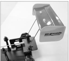
STEP 20 BEND THE WING WIRE AS SHOWN AND CUT OUT THE WING AND SIDE PLATES ( YOU MAY WANT TO PAINT THEM FIRST) USE THE LAYOUT BELOW FOR BENDING THE WIRE.DRILL TWO HOLES IN THE WING AND USE THE SMALL TIE STRAPS TO ATTACH THE WIRE UNDER THE WING. PULL THEM TIGHT AND YOU WILL BE ABLE TO ADJUST YOUR WING POSITION FORWARD AND BACK .YOU CAN ALSO CHANGE THE WIRE BENDS TO INCREASE OR DECREASE THE WING ANGLE. THE WING HAS PROTECTIVE FILM ON IT.
