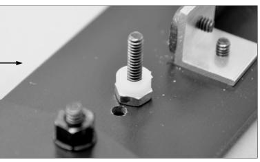
STEP 8 PRESS THE STEPPED SPACER INTO THE LARGE HOLE IN THE 5235 BELLCRANK AND SLIDE IT OVER THE LONG SCREW AND RETAIN WITH THE SMALL METAL LOCK NUT. TIGHTEN IT JUST ENOUGH THAT THE BELLCRANK ROTATES EASILY.INSTALL A STEERING LINK IN THE FRONT HOLE ON EACH SIDE OF THE BALLCRANK.
