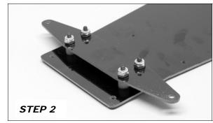
**STEP 2** INSTALL THE FRONT AXLE PLATE ON THE SCREWS AND RETAIN WITH FOUR LOCKNUTS.
