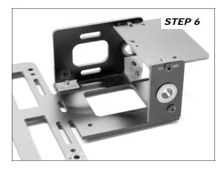
STEP 6 PRESS THE OTHER BUSHING INTO THE AXLE MOUNT. SLIDE ONE TAB ON THE SWITCH PLATE INTO THE SLOT IN THE MOTOR MOUNT, AND THE AXLE MOUNT ONTO THE OTHER TAB, AND ATTACH THE AXLE MOUNT TO THE CHASSIS WITH AN ANGLE BRACKET AND TWO 1/4" SCREWS. INSTALL 1/4" SCREWS INTO THE SLOT IN THE MOTOR AND AXLE MOUNT TO HOLD THEM TO THE SWITCH PLATE.
