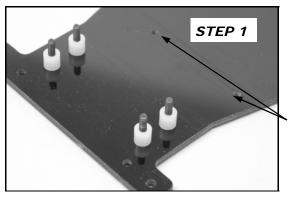
**STEP 1** REMOVE THE CHASSIS FROM BAG 1. OPEN BAG 2. INSERT FOUR 5/8 LONG SCREWS IN THE FOUR HOLES NEAR THE FRONT OF THE CHASSIS AND ADD A 1/4" SPACER ON EACH ONE, PLUS A THIN ONE ON THE FRONT TWO.
