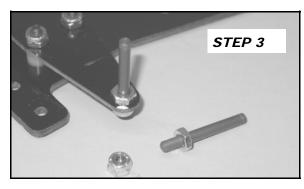
**STEP 3** OPEN THE KINGPIN BAG (INSIDE BAG 2) INSTALL A THIN NUT ON EACH KINGPIN, INSERT IT INTO THE END OF THE FRONT AXLE PLATE, ADD A LOCKNUT AND TIGHTEN, REPEAT FOR THE OTHER SIDE.
