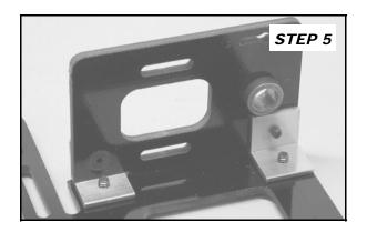
STEP 5 OPEN BAG 3 . PRESS AN OILITE BUSHING INTO THE OUTSIDE OF THE MOTOR MOUNT. ATTACH THE MOUNT TO THE CHASSIS WITH TWO ANGLE BRACKETS. NOTE THAT THE FRONT SCREW IS A FLAT HEAD AND GOES IN FROM THE INSIDE. INSTALL ALL FOUR SCREWS , THEN TIGHTEN.
