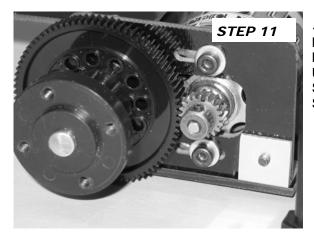
STEP 11 OPEN BAG 9 INSTALL THE PINION GEAR ONTO THE MOTOR YOU HAVE CHOSEN. INSTALL THE MOTOR WITH TWO M3 SCREWS AND WASHERS. MAKE SURE THE PINION IS LINED UP WITH THE AXLE GEAR, ADJUST THE MOTOR SO THERE IS A SMALL AMOUNT OF PLAY IN THE GEARS, AND TIGHTEN THE SCREWS. TURN THE AXLE A COUPLE OF TIMES TO RECHECK.
