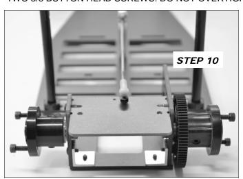
SUGGESTION: TIGHTEN THE SETSCREWS LIGHTLY TO MAKE A MARK ON THE AXLE, THEN REMOVE THE HUBS AND GRIND OR FILE A FLAT SPOT ON THE AXLE FOR THE SETSCREW TO HIT. THEN THEY WILL HOLD WITH LESS TIGHTENING.
