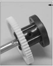
—STEP 8 INSTALL THE GEAR AND HUB ONTO THE AXLE WITH TWO SET SCREWS. ONE OF THE SET SCREWS NEEDS TO LINE UP WITH THE DRILLED INDENT IN THE AXLE. LINE IT UP AS SHOWN, THEN SLIDE THE HUB ON AND TIGHTEN THE SETSCREW. IT WILL GO BELOW THE SURFACE OF THE HUB IF THE SETSCREW IS IN THE SLOT. ADD THE OTHER SETSCREW AND TIGHTEN BOTH EVENLY TO AVOID WARPING THE HUB.
