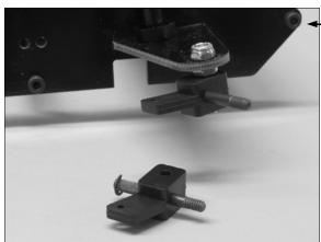
LSTEP 6 PRESS A STUB AXLE IN EACH STEERING BLOCK, ADD AN E-CLIP AND PRESS IT IN THE REST OF THE WAY. LUBE EACH KINGPIN WITH SILICONE LUBE OR LIGHT OIL, INSTALL THE STEERING BLOCK AND RETAIN WITH AN E-CLIP. INSTALL BOTH WITH THE AXLE OUT AND THE ANGLED PORTION OF THE BLOCK TO THE REAR.
