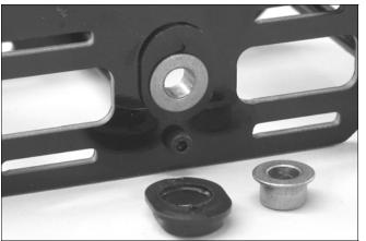
**STEP 5** OPEN BAG L1B STEERING PARTS. THREAD ONE 7206 PLAIN NUT (THIN ONES) ON EACH 5377 KINGPIN (THE PLAIN ONES WITH THE LONGER THREADS). INSERT THEM THROUGH THE ENDS OF THE FRONT AXLE PLATE AND RETAIN WITH A 7207 LOCKNUT ON EACH ONE.
