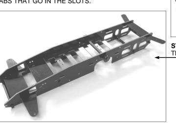
**STEP 4** INSTALL THE FRONT BUMPER UNDER THE FRONT -AXLE PLATE WITH THE TWO 1/4" CAP SCREWS (SHORTEST) SET THE CHASSIS ON YOUR TABLE TO SEE IF IT SITS FLAT. IF NOT, HOLD IT ON BOTH ENDS AND TWIST IT, THEN RE-CHECK.
