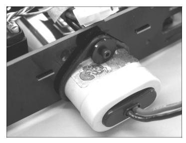
**STEP 16** IF YOU ARE USING A NICAD OR NIMH STICK BATTERY PACK, YOU CAN MOUNT IT ACROSS THE CHASSIS IN FRONT OF THE MOTOR AND USE THE O-RINGS PROVIDED TO HOLD IT IN PLACE. IF YOU ARE GOING TO RUN OVAL, YOU CAN ATTACH A PIECE OF SCRAP PLASTIC ON TOP OF THE BATTERY PACK TO KEEP IT FROM SLIDING SIDEWAYS IN AN ACCIDENT OR TO KEEP IT OFFSET TO THE INSIDE. IF YOU ARE USING A LIPO PACK YOU CAN MOUNT IT BETWEEN THE FRAME SIDES AS FAR FORWARD. OR
