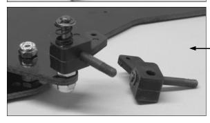
**STEP 5** LUBE EACH KINGPIN WITH A SMALL AMOUNT OF GREASE OR SILICONE LUBE. SLIDE A STEERING BLOCK ON EACH ONE, ADD A SPRING, THEN THE STEEL WASHER, AND RETAIN WITH AN E-CLIP ON EACH ONE.
