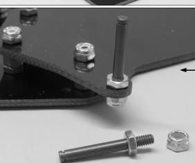
STEP 2 INSTALL THE A-ARMS AS SHOWN AND RETAIN WITH LOCKNUTS. \_\_\_\_ TIGHTEN THEM UNTIL THE A-ARMS TOUCH THE TUBING. YOU CAN ADJUST THEM LATER TO KEEP THE TIRE WEAR EVEN.
