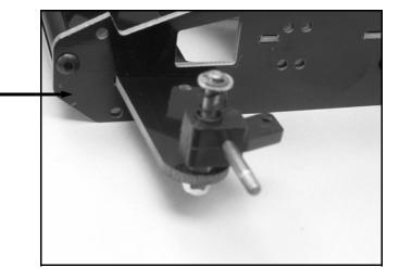
**STEP 10** INSTALL YOUR SERVO SAVER ON THE SERVO AND ATTACH THE SERVO UNDER THE SERVO PLATE WITH FOAM TAPE PROVIDED. GET THE SERVO SAVER AS CLOSE TO THE CENTER AS POSSIBLE. MAKE SURE TO WIPE THE SERVO AND SERVO PLATE WITH A DRY CLOTH BEFORE APPLYING THE TAPE. **STEP 11** INSTALL THE STEERING LINKAGE FROM BAG H3. INSTALL A LONG LINK IN EACH STEERING BLOCK AND TWO SHORT ONES IN THE SERVO SAVER. USE THE COL-LARS AND SET SCREWS TO ATTACH THE RODS TO-GETHER AFTER ALIGNING THE STEERING.
