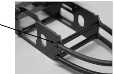
**STEP 6** USE TWO 1/2" CAP SCREWS AND THE 1/2" NY-LON SPACER TO ATTACH THE REAR BARS TOGETHER.
