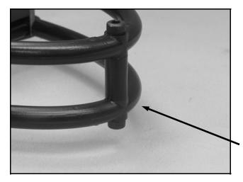
**STEP 7** OPEN THE STEERING BAG FROM BAG H1 AND THREAD A JAM NUT ON EACH 5377 KINGPIN, IN-SERT INTO EACH END OF THE FRONT AXLE PLATE, AND ADD A 7207 LOCKNUT ON EACH ONE.
