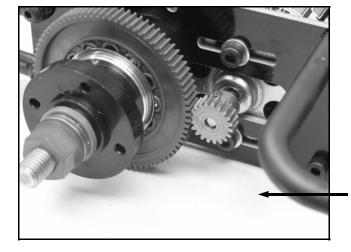
**STEP 16** INSTALL THE MOTOR YOU HAVE PURCHASED WITH M3 SCREWS AND WASHERS FROM BAG H3. INSTALL THE GEAR WITH THE SETSCREW AND MAKE SURE IT LINES UP WITH THE DIFF GEAR. SLIDE THE MOTOR BACK UNTIL YOU HAVE A VERY SMALL AMOUNT OF PLAY BE-TWEEN THE GEARS. TIGHTEN THE MOTOR SCREWS , TURN THE AXLE A COUPLE OF TIMES, CHECK THE GEAR MESH , AND READJUST IF NECESSARY.
