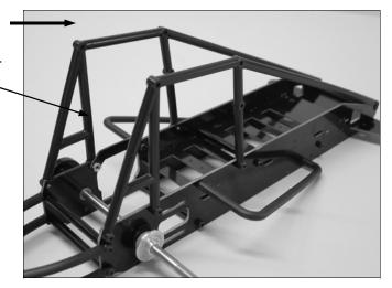
**STEP 21** USE 1/2" BUTTON HEAD SCREWS AND THREE CHASSIS SPACERS TO ATTACH THE TWO SIDES OF THE ROLL CAGE TOGETHER. THE TOP TWO WILL ALSO BE USED TO HOLD THE WING MOUNTS ON LATER.
