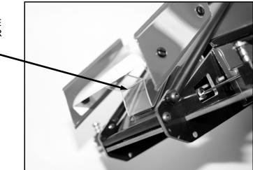
**STEP 27** INSTALL THE REAR WING TO THE ROLL CAGE WITH THE SCREWS THAT ATTACH THE CHASSIS BRACES . YOU CAN SLOT THE HOLES IN THE MOUNTS FOR EASY REMOVAL, BUT THE WING MAY NOT STAY ON AS WELL IN A HARD CRASH.
