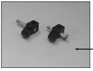
**STEP 9** LUBE EACH KINGPIN, SLIDE THE STEERING BLOCK ON, ADD A 5228 SPRING , WASHER , AND E-CLIP.
