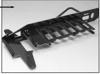
**STEP 4** SLIDE THE LEFT CHASSIS OVER THE PARTS AND ATTACH WITH 3/8 CAP SCREWS (BUTTON HD. ON FT.).SET THE CHASSIS ON YOUR TABLE TO MAKE SURE IT SITS FLAT. IF NOT, HOLD BOTH ENDS AND TWIST TO CORRECT. CHECK 1 IT AGAIN AFTER INSTALLING THE REAR BARS AND CAGE. **STEP 5** ATTACH THE REAR BARS AND CHASSIS SPACERS TO THE REAR OF THE CHASSIS WITH FOUR 1/2" BUTTON HEAD SCREWS.
