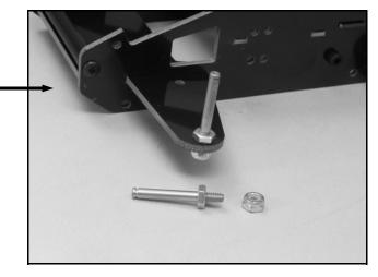
**STEP 8** PRESS A 5364 STUB AXLE INTO EACH 5351 STEERING BLOCK AND RETAIN WITH A 5221 E-CLIP.
