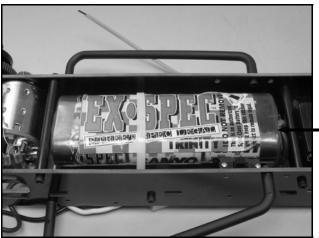
**STEP 20** OPEN BAG H1A. MOUNT THE ROLL CAGE SIDES TO THE CHASSIS WITH 3/8 BUTTON HEAD SCREWS. USE THE 1/4" (SHORT) SCREWS IN THE FRONT HOLES. ADD THE JAM NUT FROM BAG A AT THE REAR OF THE TIE BAR.
