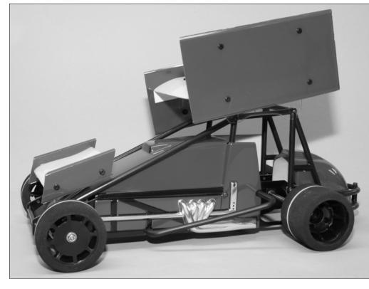
STEP 28 PRESS THE BUSH-INGS FROM BAG H3 INTO EACH SIDE OF EACH FRONT WHEEL FROM BAG L4. LUBE THE FRONT AXLES WITH LIGHT OIL AND INSTALL THE FRONT WHEELS. ADD LOCK-NUTS FROM THE STEERING BAG TO HOLD THEM ON. TIGHTEN THEM LIGHTLY. THEN BACK THEM OFF UNTIL THE WHEELS SPIN FREELY. INSTALL THE REAR TIRES FROM BAG L5 TO THE REAR HUBS WITH TWO 3/8 CAP SCREWS EACH FROM THE DIFF BAG. THE TIRES IN YOUR KIT MAY VARY FROM THE ONES SHOWN. THEY WILL BE OF THE SAME OR BETTER QUALITY.
