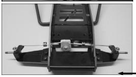
MAKE SURE TO WIPE THE SERVO AND THE FRONT AXLE PLATE WITH A DRY CLOTH BEFORE APPLYING THE SERVO TAPE.
