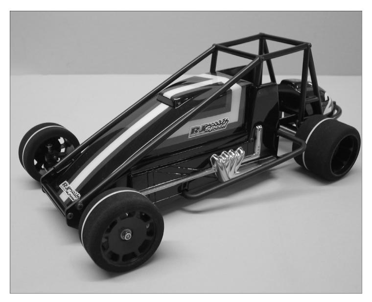
**STEP 28** PRESS THE BUSHINGS FROM BAG H3 INTO EACH SIDE OF EACH FRONT WHEEL FROM BAG L4. LUBE THE FRONT AXLES WITH LIGHT OIL AND INSTALL THE FRONT WHEELS. ADD LOCKNUTS FROM THE STEERING BAG TO HOLD THEM ON. TIGHTEN THEM LIGHTLY, THEN BACK THEM OFF UNTIL THE WHEELS SPIN FREELY.
