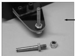
**STEP 8** OPEN THE STEERING BAG FROM BAG H1 AND THREAD A JAM NUT ON EACH 5377 KINGPIN, INSERT INTO EACH END OF THE FRONT AXLE PLATE, AND ADD A 7207 LOCKNUT ON EACH ONE.
