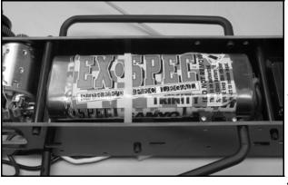
STEP 20 INSTALL YOUR BATTERY PACK UNDER THE RADIO TRAY WITH A TIE STRAP. YOU SHOULD HAVE ROOM TO MOUNT YOUR SWITCH NEXT TO IT WITH SERVO TAPE SO YOU CAN TURN THE CAR ON AND OFF WITHOUT REMOVING THE BODY. YOU CAN ALSO MOUNT THE SWITCH NEXT TO THE SERVO IF YOU HAVE ROOM.
