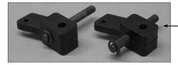
**STEP 6** LUBE EACH KINGPIN, SLIDE THE STEERING BLOCK ON, ADD A 5228 SPRING, WASHER, AND E-CLIP.
