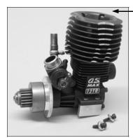
STEP 10 OPEN BAG 12 INSTALL YOUR CLUTCH ONTO YOUR ENGINE AND ATTACH THE ALUMINUM ENGINE MOUNTS TO THE ENGINE WITH FOUR 1/4" CAP SCREWS AND THIN STEEL WASHERS. IT MIGHT BE A GOOD IDEA TO USE A SMALL AMOUNT OF REMOVABLE LIQUID THREAD LOCK TO PARTS THAT WILL-CONNECT TO THE ENGINE . IF YOU ARE USING A PULLSTART ENGINE , YOU MAY NEED OUR #5145 SPACER AND SCREW KIT TO RAISE THE ENGINE TO CLEAR THE PULLSTART.
