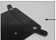
STEP 2A INSTALL THE REAR BODY MOUNT NEAR THE REAR OF THE CHASSIS WITH TWO 1/4" SCREWS AND NUTS
