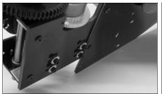
STEP 19 INSTALL THE ENGINE ON THE BOTTOM PLATE WITH FOUR 3/8" SCREWS AND THICK WASHERS.SLIDE THE AXLE ASSEMBLY THRU THE BUSHINGS AND MESH THE GEARS SO THAT THERE IS A SMALL AMOUNT OF PLAY BETWEEN THE GEARS, THEN TIGHTEN THE MOTOR SCREWS. MAKE SURE YOU HAVE THE ENGINE STRAIGHT OR THE REAR SLIGHTLY FORWARD.
