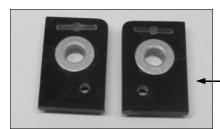
**STEP 14** PRESS AN OILITE BUSHING INTO EACH OF THE REAR AXLE MOUNTS AS SHOWN. NOTE THAT BOTH MOUNTS ARE ALIKE AND THE ROUNDED TOP SIDE OF EACH ONE WILL GO TO THE REAR OF THE CAR. THE LARGE PART OF THE BUSHING SHOULD BE TO THE OUTSIDE WHEN YOU MOUNT THEM.
