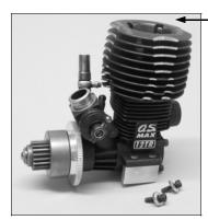
STEP 18 OPEN BAG 12 INSTALL YOUR CLUTCH ONTO YOUR ENGINE AND ATTACH THE ALUMINUM ENGINE MOUNTS TO THE ENGINE WITH FOUR 1/4" CAP SCREWS AND THIN STEEL WASHERS. IT MIGHT BE A GOOD IDEA TO USE A SMALL AMOUNT OF REMOVABLE LIQUID THREAD LOCK TO PARTS THAT WILL-CONNECT TO THE ENGINE . IF YOU ARE USING A PULLSTART ENGINE , YOU MAY NEED OUR #5145 SPACER AND SCREW KIT TO RAISE THE ENGINE TO CLEAR THE PULLSTART.
